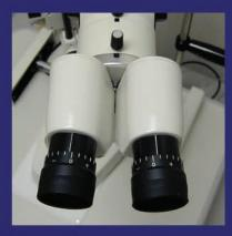
Galilean optical system incorporates an 8 degree convergence to enhance comfort and ease of image fusion
